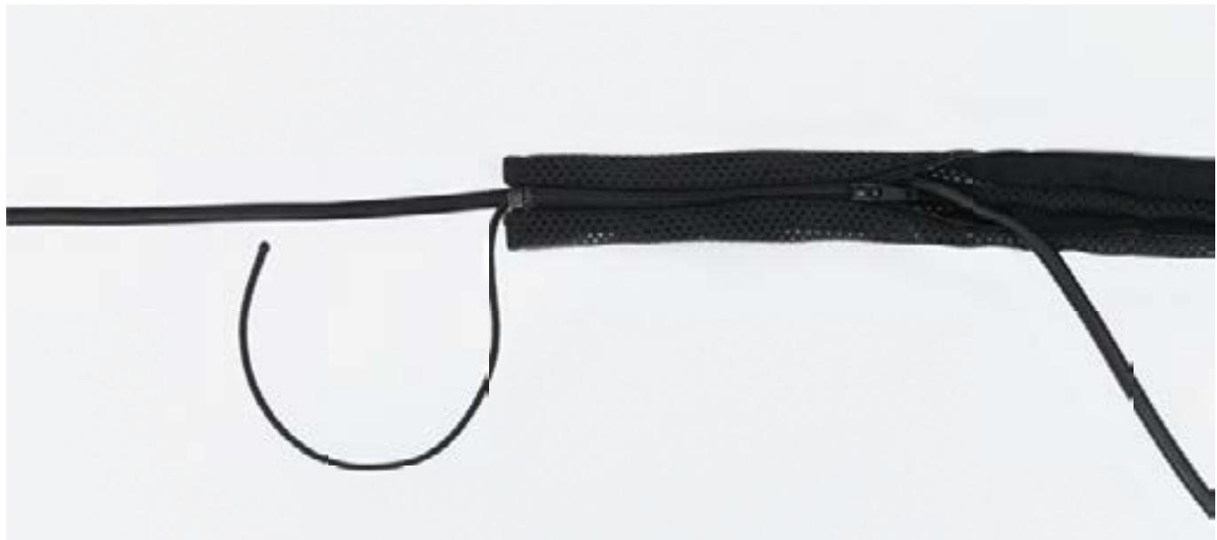
Cable net Made of polyester, the cable net is 150 cm long and fitted with 4 zip fasteners. It can hold up to 6 cables and is affixed with cord ties, e.g. to the cable basket. Colour: basic dark
